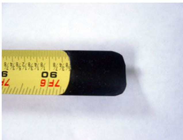
Fig. 3 - Tips of the elements, rounded & coated
